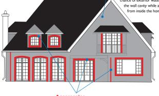
TYPAR offers three flashing options to ensure seal integrity around doors, windows, and other exterior rough openings. TYPAR® Flashing RA offers affordable, best-in-class performance. TYPAR® Flashing BA is our premium butyl-based flashing. TYPAR® Flashing Flex is butyl-based and perfect for sealing around arched windows. TYPAR® Construction Tape is a strong, polypropylene film, coated with a powerful all-weather acrylic adhesive that seals out the elements.
