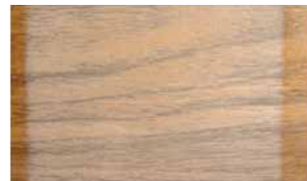
Sample 2 NOT Protected with Acrylic Topcoat 11.62 delta-E color change
